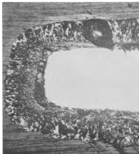
Fig. 12. Photomicrograph of section of specimen, attacked in sulfur vapor at 500°C (vessel with liquid sulfur at 230°C), after a 48-hr aging in hydrogen at a pressure slightly above 1 atm. Note EPON resin around metal contour as a result of scale spalling. Magnification, 200 \times before reduction for publication.
