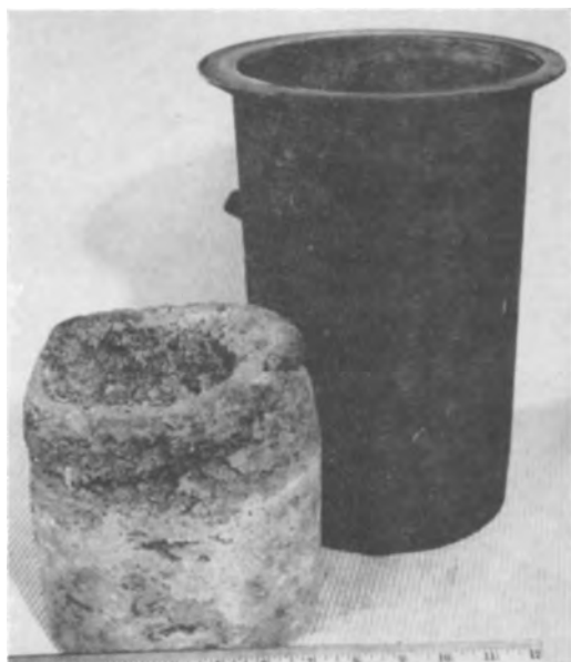
Fig. 1. Calcium reduced thorium oxide reduction cake. Type 446 stainless steel reduction vessel.
