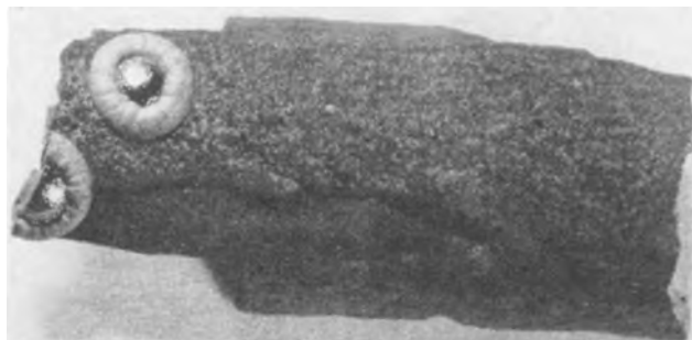
Fig. 5. Fragment of iodide boron made at 900°C
