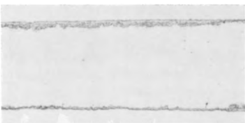
Fig. 3. 12.8% Cr oxidized 5 min, 1000°C; equilibrated 65 hr argon, 1000°C. Note transition scale: partly internal oxide, partly surface oxide. Magnification 100X before reduction for publication.
