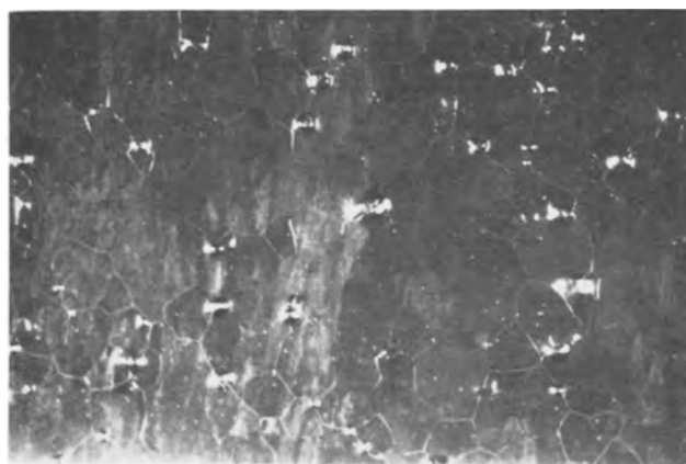
Fig. 4. Surface of aluminum oxidized in 0.1 atm water vapor at 600°C. Magnification 25X before reduction for publication.
