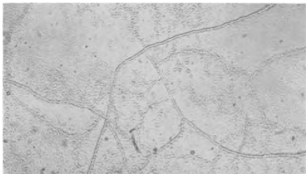
Fig. 10. Optical photograph of (100) surface shown in Fig. 8B. Magnification 200X before reduction for publication.
