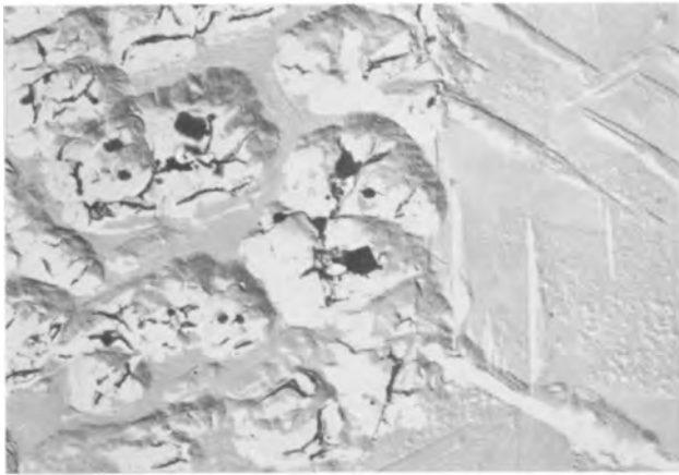
Fig. 6. Blister-like cracks appearing in grain after prolonged oxidation at 600°C. Annealed 1 hr at 1200°C; oxidized 15 min at 600°C; indirect replica. Magnification 6900X before reduction for publication.
