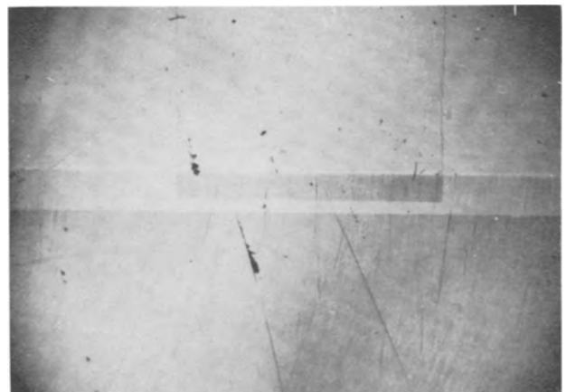
Fig. 3. Photomicrograph of an oxide masked double-diffused wafer. The junctions have been exposed by bevel lapping and polishing at an angle of about 5° and staining the p regions.
