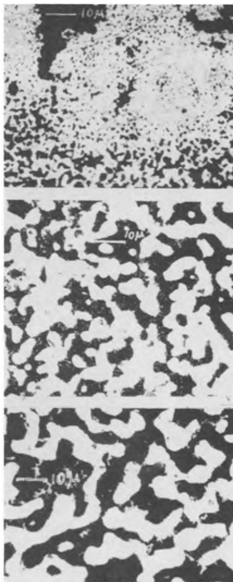
Fig. 8. Structures of two-phase layers obtained on Cu-Au alloys ( N_{Au} = 0.33 , as-received). (a) (top) Sample sulfidized at 500°C for 16 min; (b) (center) sample sulfidized at 500°C for 20 min and annealed in sulfur vapor at 700°C for 16 min; (c) (bottom) sample sulfidized at 700°C for 4 min.
