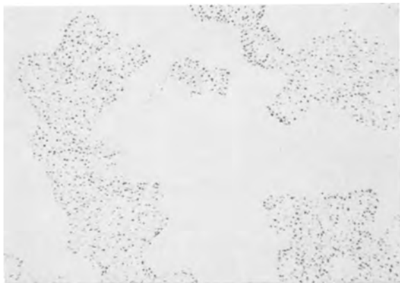
Fig. 8. Low magnification of nodular growths on tantalum surface oxidized at 700°C. Annealed 16 hr at 1200°C; oxidized 6-10 sec at 700°C. Magnification 500X before reduction for publication.
