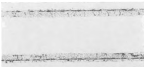
Fig. 2. 9.94% Cr oxidized 1½ hr, 1000°C; equilibrated 64 hr argon, 1000°C. Note layer of internal spinel. Magnification 100X before reduction for publication.
