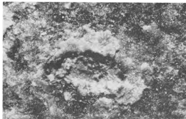
Fig. 8. Characteristic appearance of the metal surface after second breakaway, oxidized at 450°C for 47 hr. Magnification 200X before reduction for publication.
