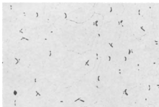
Fig. 2. Arc melted thorium button, run No. 58, bright field, 200X, 0.37% \text{ThO}_2 .
