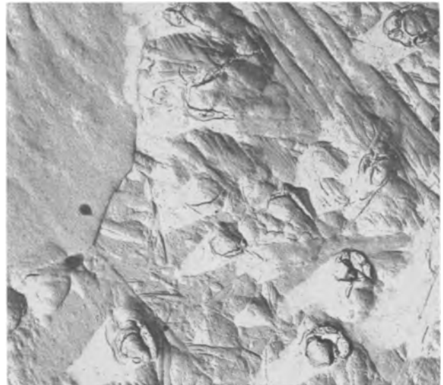
Fig. 5. Electron micrograph of the surface of a Ta specimen oxidized for 10 hr at 515°C. Direct carbon replica, preshadowed with gold-manganin. 12,500 X
