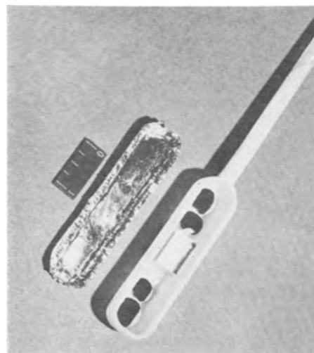
Fig. 1. Modified closed box showing quartz boat containing Pt source box and polished Si wafers. Formed Pt gasket is shown at left.
