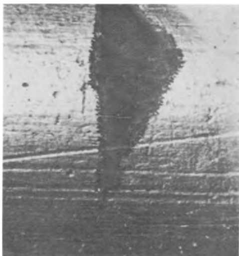
Fig. 4. Copper sulfide growth from scratch in nitrocellulose lacquer on copper after 24 hr over sulfur at 60^\circ . Area shown: 7.8 \text{ mm}^2 .
