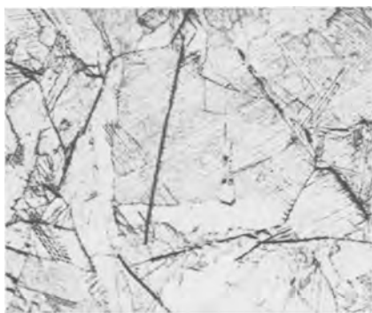
Fig. 7. L-170BC-gamma quenched. Chromic acid etch, VHN-382, 30 kg. Magnification 500X before reduction for publication.
