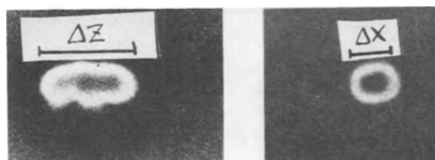
Fig. 5(a) (left). shows the central spot in Fig. 1, enlarged 35 times. It spreads along the direction of the field. Fig. 5(b) (right). shows the cross section of the undistorted incident beam; it is nearly circular.
