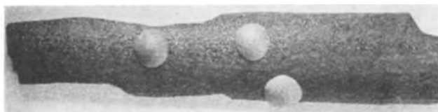
Fig. 4. Fragment of iodide boron made at 900°C
