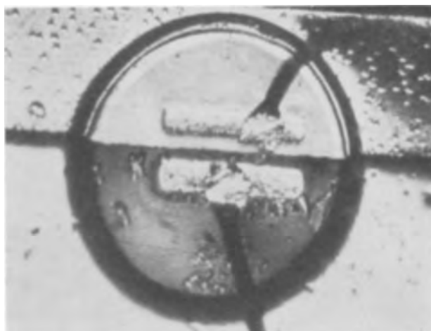
Fig. 4. Photomicrograph of completed unit showing the gold stripes and bonded leads.
