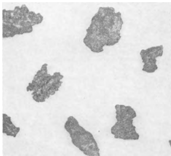
Fig. 2. Thorium metal particles (+10 mesh) produced by electrolysis of \text{ThO}_2 in a \text{KF-ThF}_4 melt, following leach with hot aqueous aluminum nitrate.
