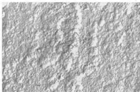
Fig. 11. L-170BC-gamma quenched and aged 400°C, 15 min, Ames etch, 16,100X—5282A.
