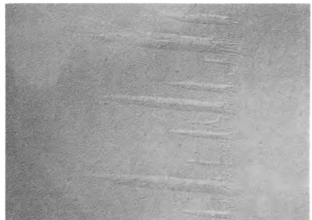
Fig. 1. Typical grain-boundary platelet growth on tantalum oxidized at low temperature. Note "bubble raft" background texture. Annealed 1 hr at 1200°C; oxidized 95 hr at 300°C; indirect replica. REF: J. V. Cathcart, R. Bakish, and D. R. Norton, This Journal, in press. Magnification 16,800X before reduction for publication.
