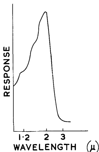
Fig. 7. Spectral response of PbTe cell H14 measured immediately after formation.
