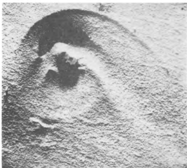
Fig. 5. Enlargement of marking caused by surface obstruction. Magnification 30X before reduction for publication.
