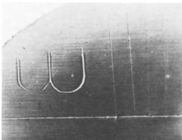
Fig. 2. Autoradiograph (5X before reduction for publication) of nickel plated on disk G which had parallel scratches in one direction. Center line average roughness of fine scratches 1.17 \mu .
