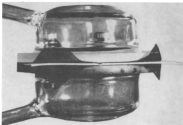
Fig. 2. Type 1 ion-exchange membrane fuel cell, active area, 25 cm 2 .
