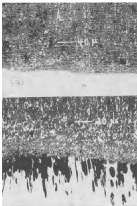
Fig. 7. Details of alloy-scale boundary of Cu-Au alloys ( N_{Au} = 0.10 ) sulfidized at 500^{\circ}\text{C} for 4 min. (a) (top) Annealed sample; (b) (bottom) as-received sample.
