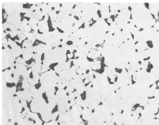
Fig. 1e. Specimen 91, —200 mesh powder ground and loaded in air, hot pressed at 2000 psi, 750°C, 5 hr.
