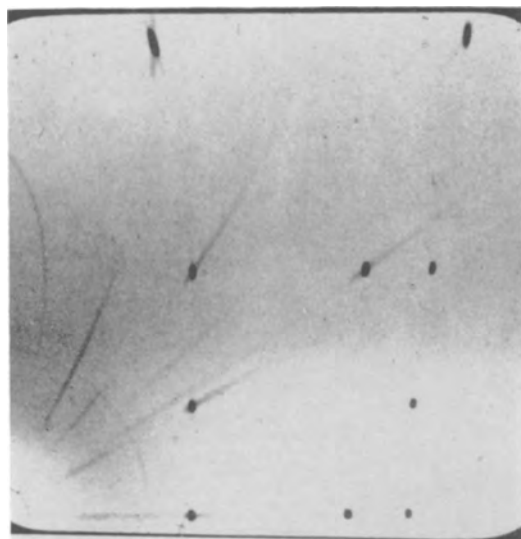
Fig. 5. X-ray diagram of hexagonal zinc sulfide single crystal rotated about the c -axis.
